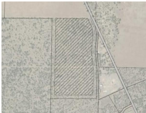
Forest Irrigation Area with an effluent disposal potential of 77 acre feet per year
