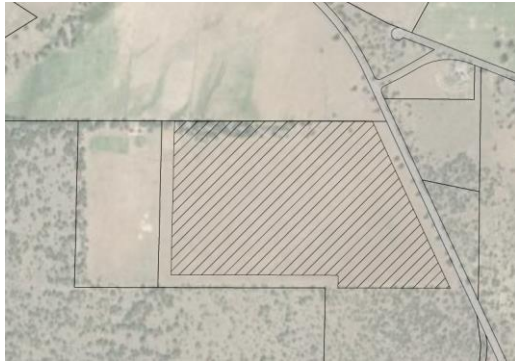
Crop irrigation with an effluent disposal potential of approximately 166acre feet per year
