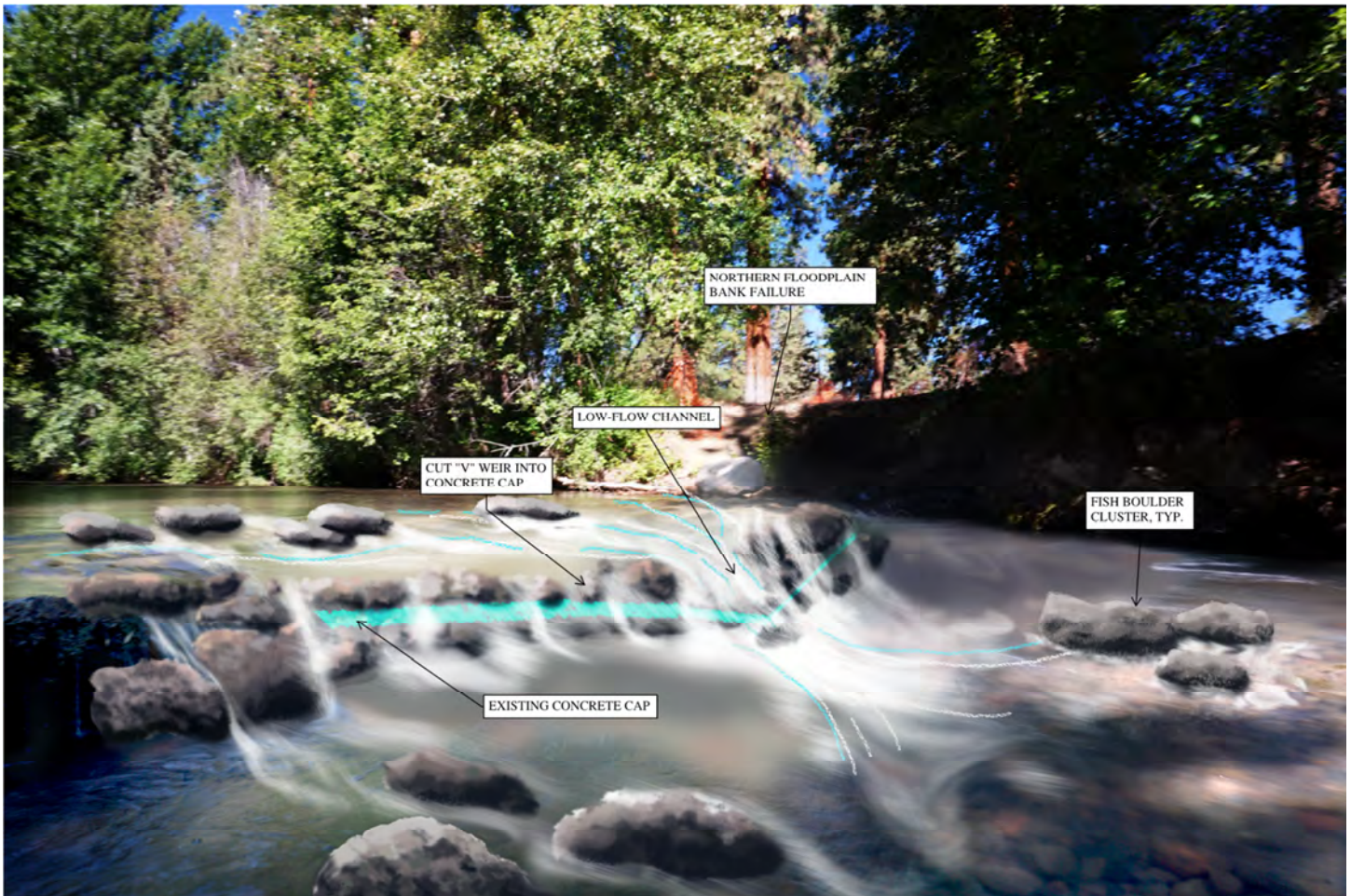
Figure 4: Photo Rendering (C. Schenider) of Example V-Shaped Notch Weir along In-Stream Concrete Cap
