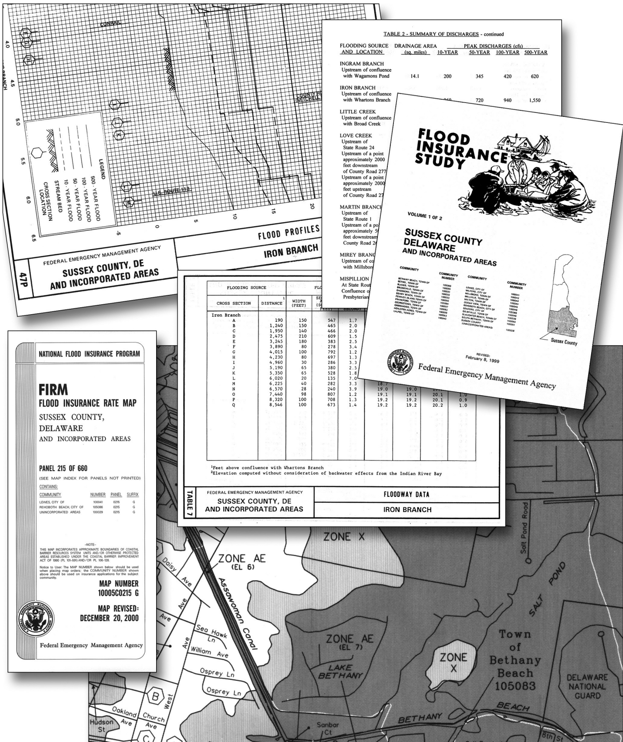
Figure 4-1. Portions of an FIS and a FIRM.
