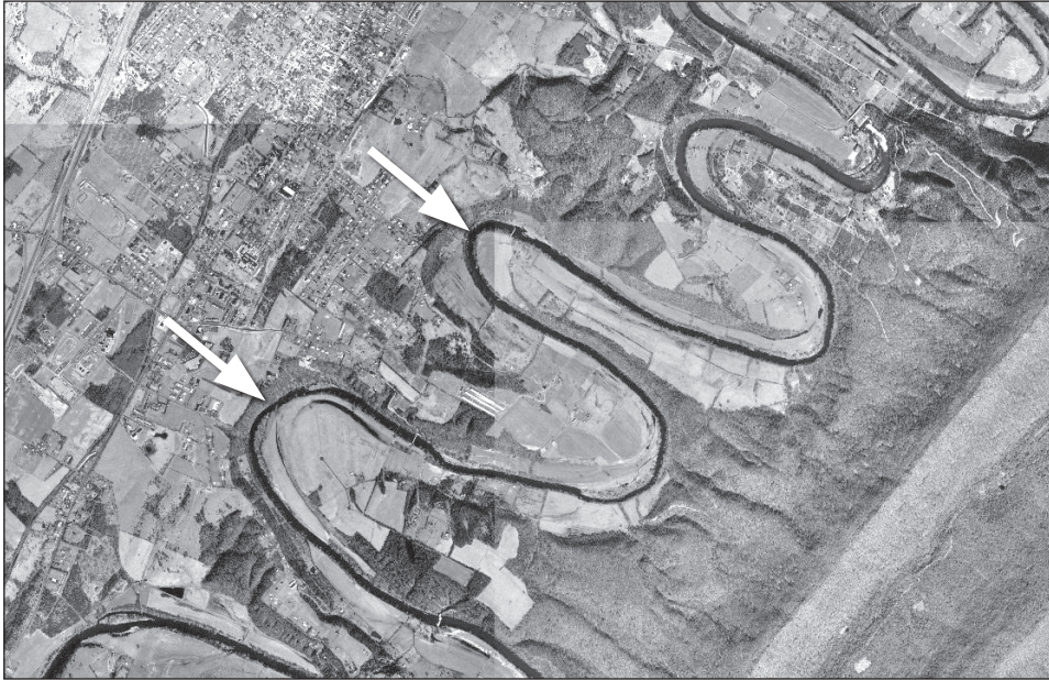
Figure C-8. Meandering stream system. Velocities are generally higher along the outer bends of streams.
